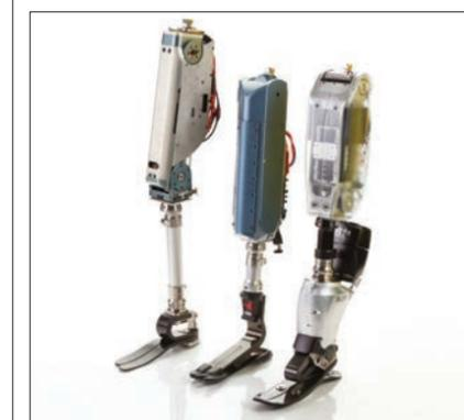
“You can say that conventional mechanical prostheses are like a bicycle and what I’m wearing is like a motorcycle—the motors actually inject mechanical energy into my walking gait, enabling me to move more efficiently,” Herr said.
