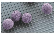
© CELLULAR INJECTION Hongkun Park is developing nanowire arrays that can inject neurons with chemicals or measure electrical activity as it develops in the cell. Here, Park's array interrogates immune system T cells.
