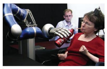
THOUGHT INTO ACTION A 4 millimeter square sensor (left) implanted in the brain of Cathy Hutchinson uses 96 electrodes to capture neural signals. A computer decodes the data, enabling Hutchinson, who has been paralyzed 15 years, to manipulate a robotic arm and give herself a drink of coffee.
