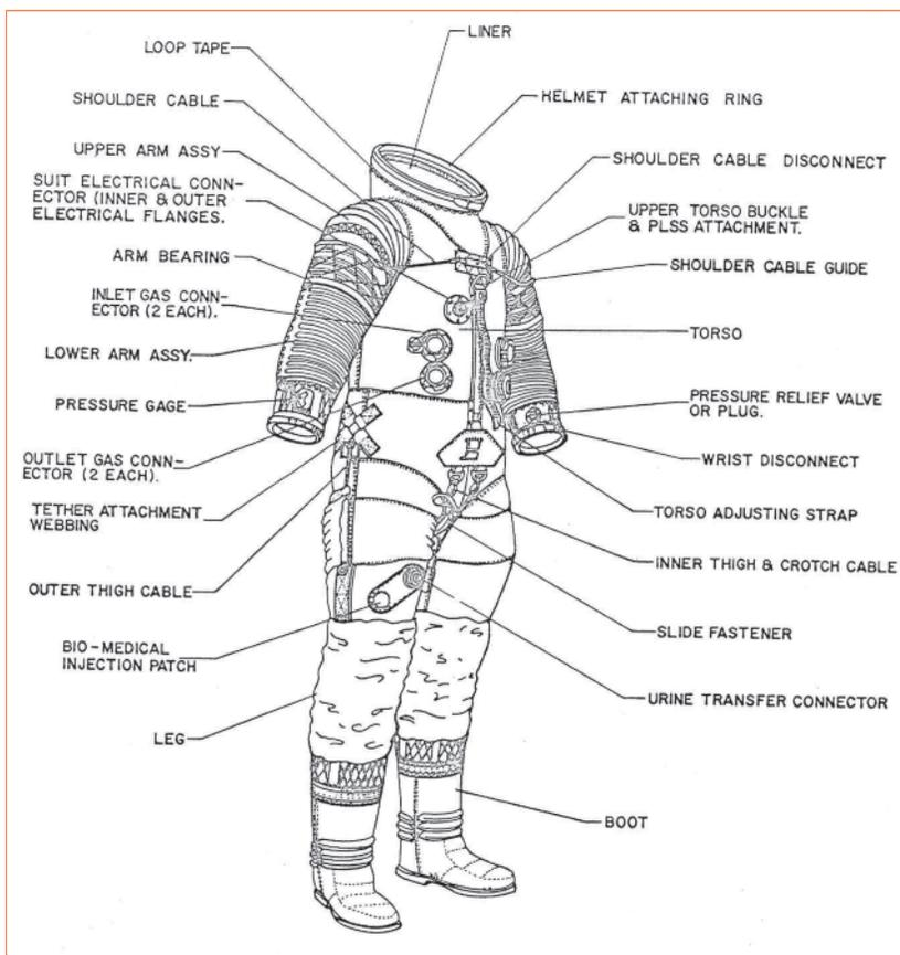
An electrical connector was provided on the torso for the pass-through of the communications system as well as biomedical signals that would be broadcast back to NASA doctors who would monitor astronauts' conditions.
