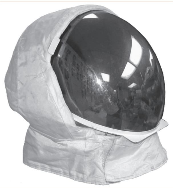
Worn over the pressure helmet was the extravehicular visor assembly or EVVA.
