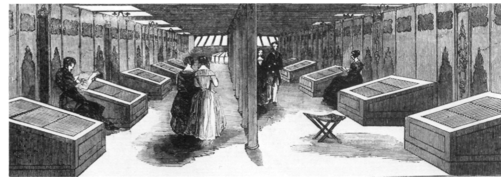
Looking aft through the original Promenade Deck of the Great Britain with staterooms or cabins ranged along each side. The box fittings gave light to the Dining Saloon below.
