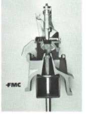
As the extractor cycle Continues, pressure increases on the citrus causing the internal portions of the fruit to be forced through the bottom plug and into the prefinisher tube. The peel is now being discharged between the upper cup and cutter. cutter.
