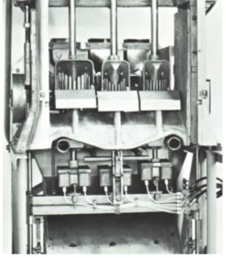
091. THE OFFICIAL STATE OF FLORIDA FRUIT TESTING EXTRACTOR for measuring fruit characteristics to determine truck load prices.
