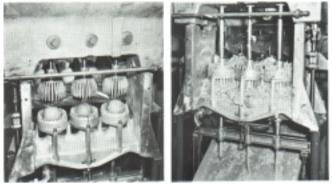
659 PROTOTYPE. Note the orifice discharge tubes at bottom which removed core, membrane and seeds from juice at the moment of extraction. 659 PROTOTYPE for grapefruit 4"-6" diameter.
