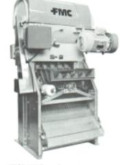
LATEST MODEL 291B. In-place cleanup & recycle peel oil recovery systems. 100 strokes/500 fruit per minute.
