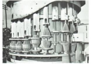
402X with covers removed. 24 heads, 20 strokes/480 fruit per minute. Note 20 finger cup with strippers.
