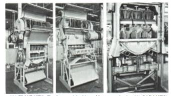
291 FRONT VIEW. The first model with positive rotary feeder. 291 BACK VIEW. The rotary feeder permitted the operating speed to increase to 75 strokes/375 fruit per minute. 491, FIRST MODEL TO USE 5" OIL RECOVERY CUPS AND ROTARY FEED. 60 strokes/180 fruit per minute.
