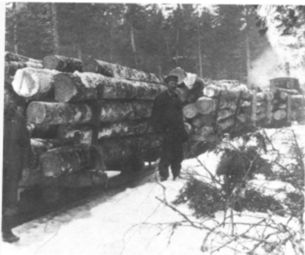
A typical log hauler crew consisted of an engineer, fireman, conductor, and the steerer. The conductor, riding close to the rear, communicated with the cab by a bell rope which ran along the sled stakes.
