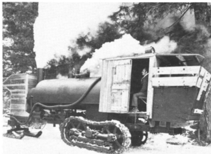
A woodburning "Lombard" (c. 1900-1910) built in Waterville, Maine. It was put into operating condition February 7, 1980 for a two-mile run—its performance was deemed "superb".
