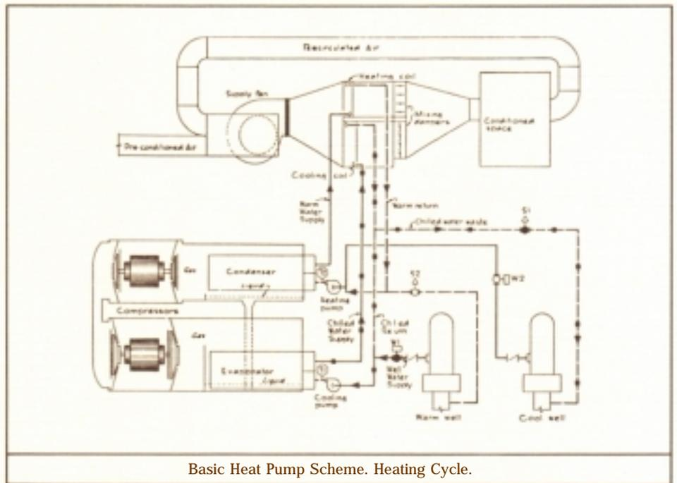
Outside air was not used for the internal or minimum cooling, inasmuch as to do so would have required equipment arrangement on each floor, encroaching on rentable floor space and would have necessitated additional complexity in automatic control.
