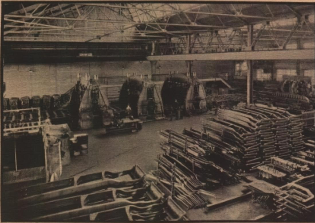
There were six presses at the starting end of the side bar manufacturing line. Besides the piercing, blanking and forming of the strip steel used, they gave the offsets (in the plane of the strip) to provide for the kick up over the rear axle and the front and rear end drops.
