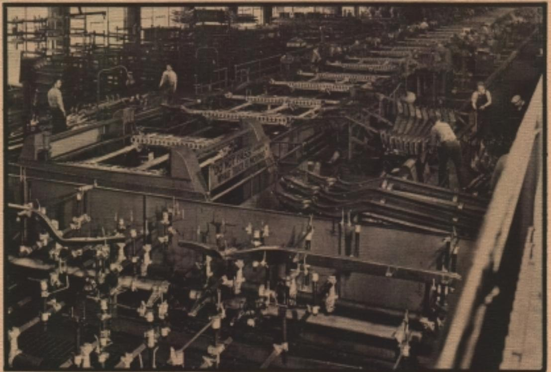
In parallel lines the left side bars, the right side bars and the different cross bars came forward from the far end of the building, receiving automatically on the way various machining and other operations. In the foreground is the part of the machine to which these sub-assemblies of bars were delivered, progressing transversely across the building. The parts were clamped together and fastened by rivets fed through compressed air tubes to the riveting guns.
