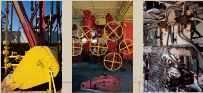
Drilling rig equipment and machinery as it appears today on Mr. Charlie. From left to right: a pulley assembly, an array of valves and the blowout preventer controls.
