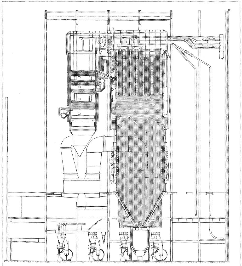
Figure 6: Supercritical pressure steam generator- side elevation
