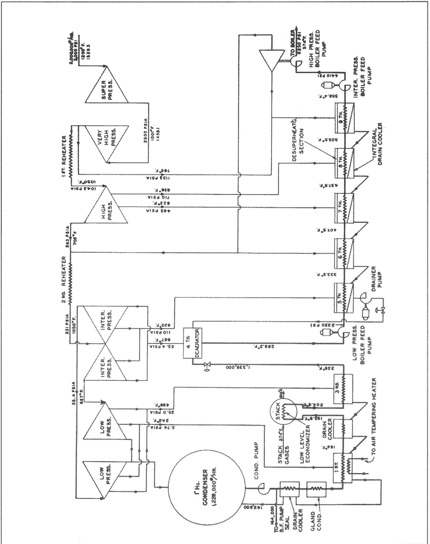
Figure 8: Single - line arrangement of feedwater heaters and pumps
