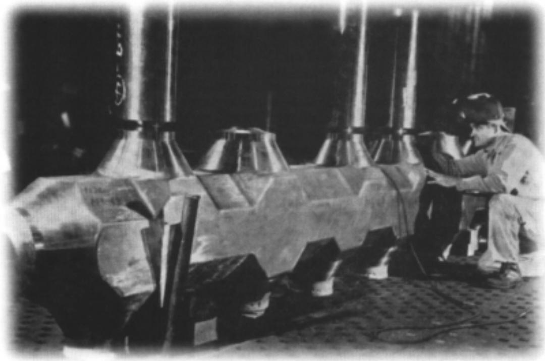
Figure 11: Weld pass between junction header and four stub ends
