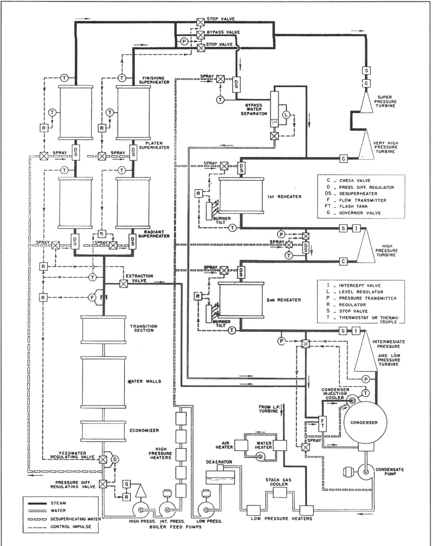
Figure 7: Simplified flow diagram, showing controls and startup-system
