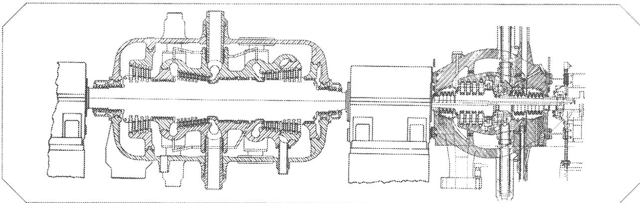
Figure 2: Cross-section of 3600 rpm turbines
