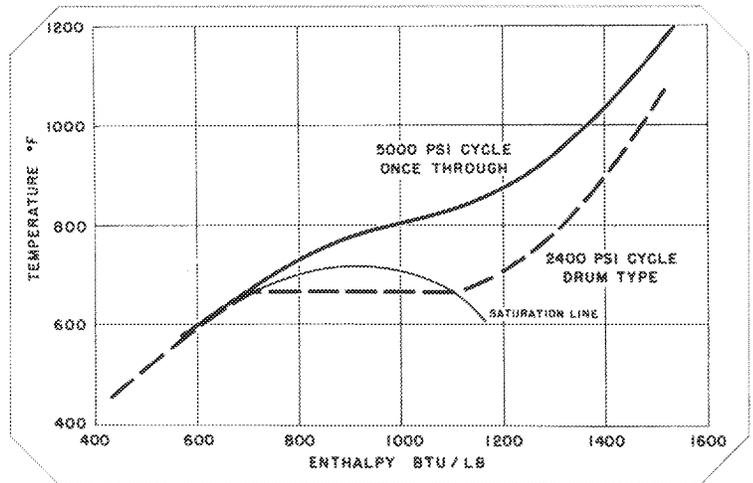
Figure 4: Temperature-enthalpy diagram
