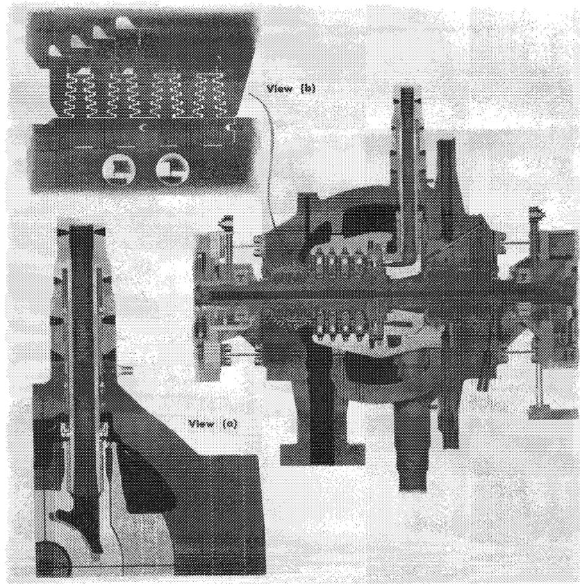
Figure 5: Longitudinal section - SP turbine element
