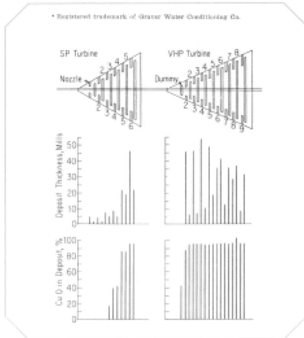
Figure 1.4: Metallic deposits in final stages of SP and all of VHP elements showing high copper content
