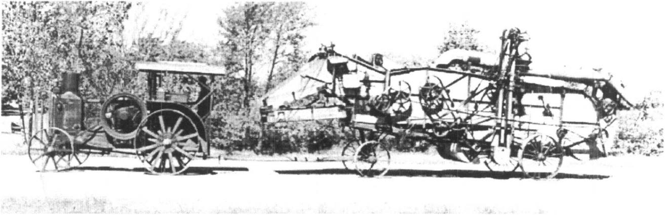
Rumely OilPull Tractor towing steel separator
