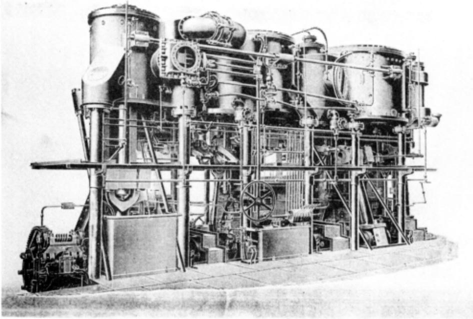
Above -- Front view, from high-pressure end, of starboard engine of U.S.S. Olympia, showing control station. Valves (all piston) were actuated by Stephenson link motion
