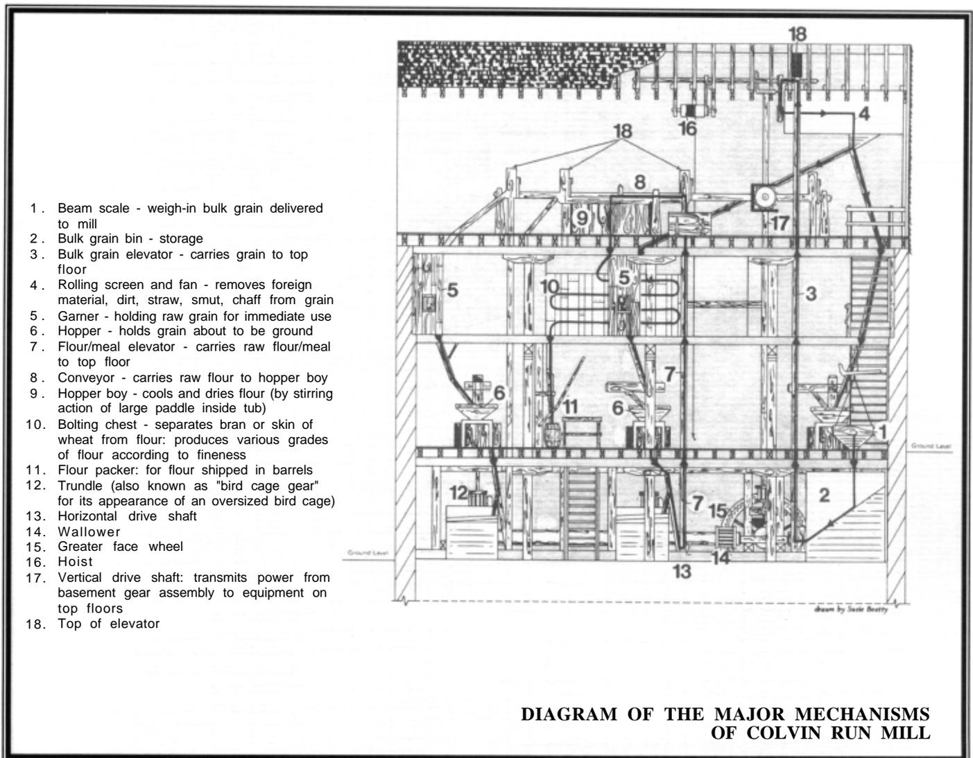
**DIAGRAM OF THE MAJOR MECHANISMS OF COLVIN RUN MILL**
