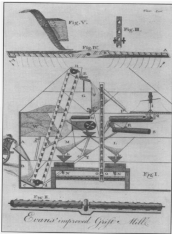
Automation required many mechanical motions and some entirely novel devices invented by Evans, including a mechanical hopper boy, a raking device used to cool flour. Colvin Run Mill exhibits the sole operating hopper boy known in the United States. In combination, Evans' milling innovations boosted
