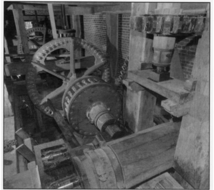
The gears transmit power from the waterwheel to all the machinery in the mill, including three shaker boxes in the basement, the three grinding stations on the first floor, the bolting chest and hopper boy on the upper floors, and the grain elevators that operate throughout the four floors of the mill.
