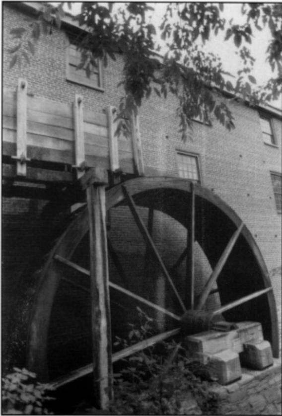
Around the outside of the wheel are sixty buckets inclined at an angle to catch water falling from the flume above. Each bucket holds approximately fifteen gallons (or 125 pounds) of water. The weight of water filling the buckets turns the waterwheel in
