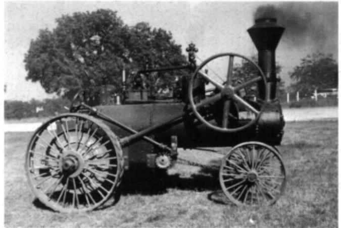
*Cooper Self-Propelled, Self-Steering Traction Engine*
