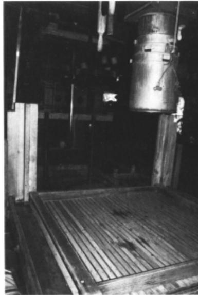
The mill featured a sophisticated method of grinding the fruit and a press capable of applying pressure at three speeds. This model, using all steel construction, was considered the finest screw cider press ever made. In the twentieth century, the hydraulic press came into widespread use. Thus, B.F. Clyde's Cider Mill is representative of the final and finest mills using the mechanical screw press.
