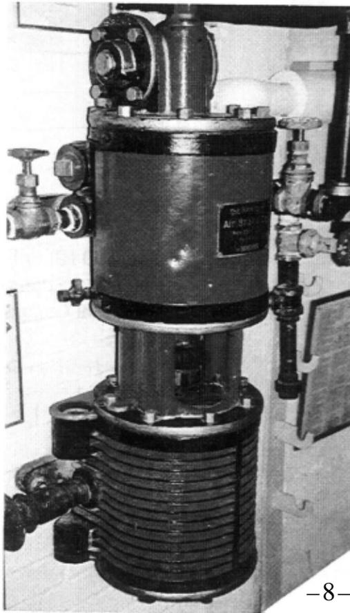
Engine #15 Locomotive Air Compressor
