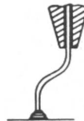
Capillary moves toward leadframe contact
