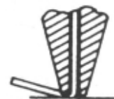
Stitch bond made on leadframe contact with edge of capillary
