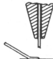
Capillary retracts as wire is clamped and broken
