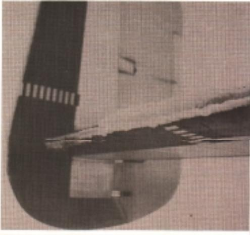
*Severe icing on B-24 stabilizer (no deicing protection).*
