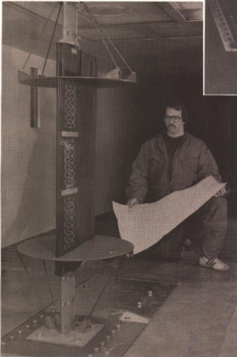
*Unique icing problems associated with the helicopter are resulting in many IRT tests by government and industry. The test of the rotor section shown here was to evaluate proposed electrothermal deicing designs.*
