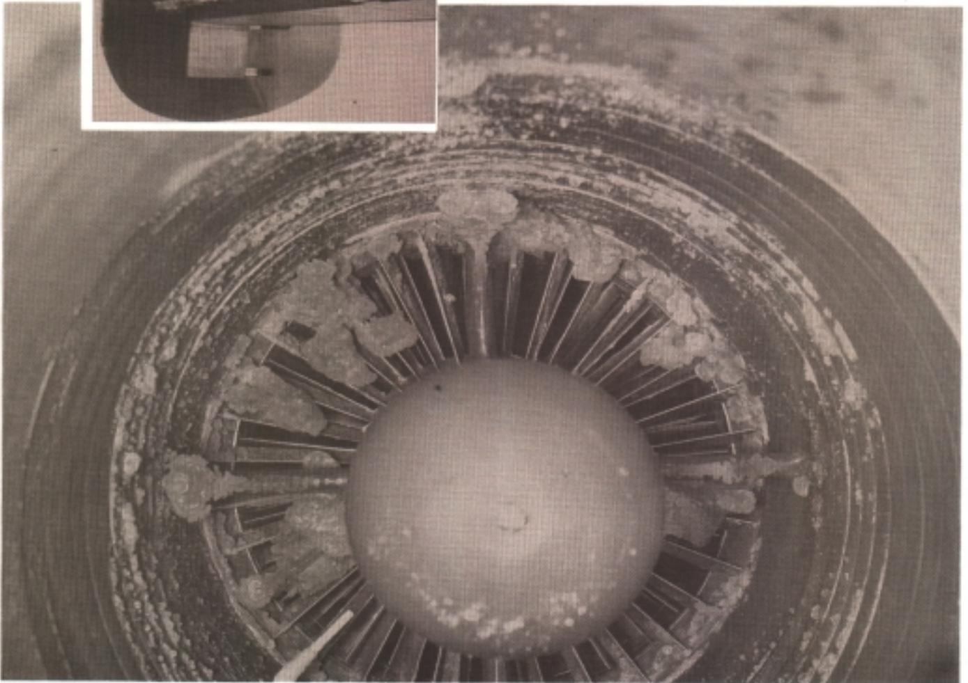
*Ice on inlet guide vanes of an early jet engine (no deicing protection)*
