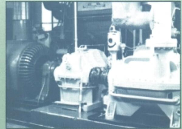
1,500 hp centrifugal compressor driven by original wound-rotor induction motor through step-up gears. A one-meter stick appears in this photograph.
