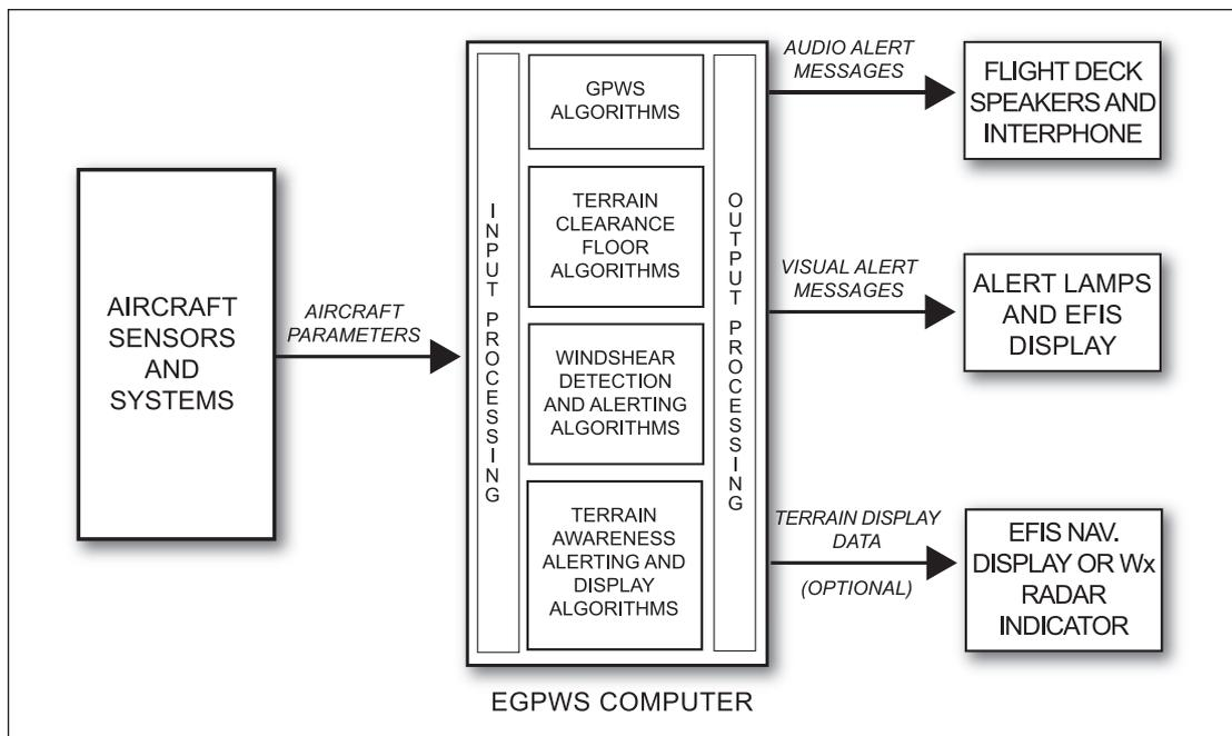
Figure 2-- Enhanced GPWS (EGPWS) BLOCK DIAGRAM.
