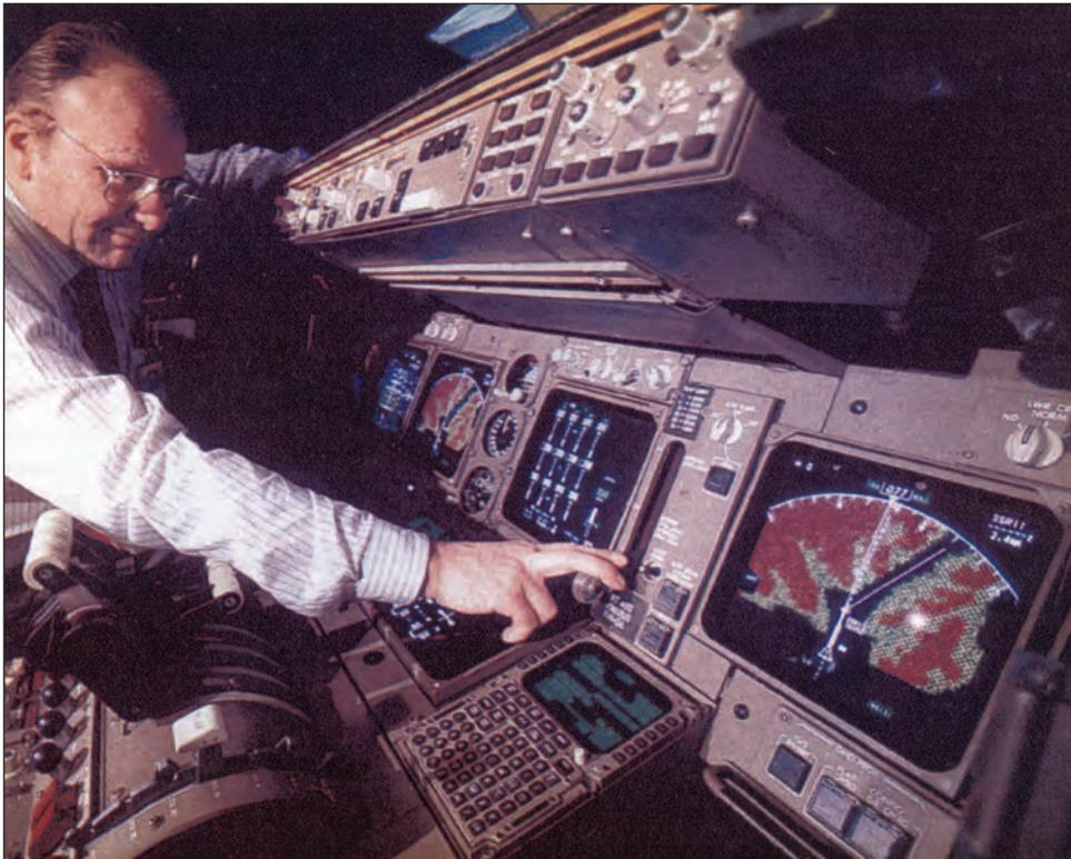
*Figure 3-- A cockpit with EGPWS/terrain-weather radar display.*
