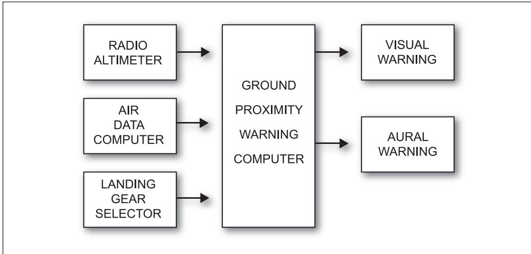
*Figure 1 -- 1967 GPWS Computer System Block Diagram.*
