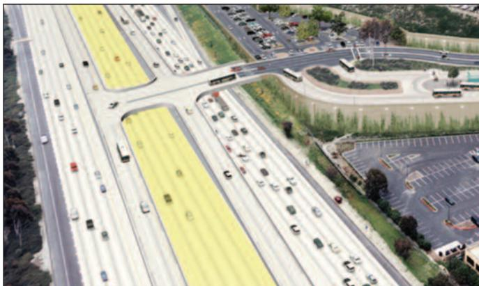
*The four center lanes on this section of I-15 are reconfigured by moveable barrier.*
