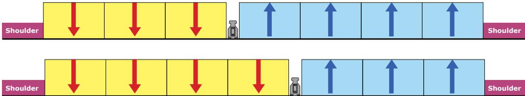
*The median barrier can be adjusted multiple times per day to meet peak demand.*
