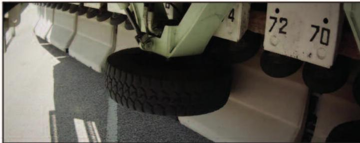
*The barriers are passed through the conveyor underneath the BTM.*
