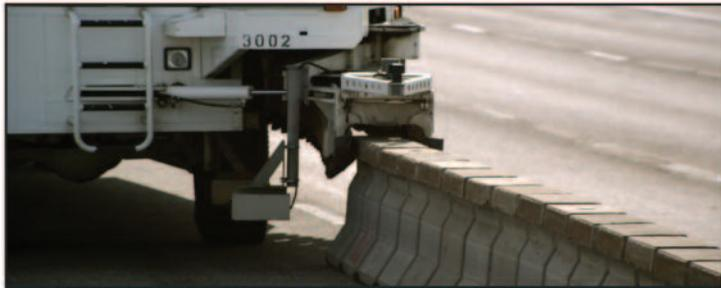
*The BTM lifts the barriers using a conveyor wheel system.*
