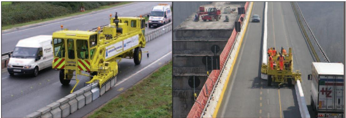
*Moveable barrier is transferred under traffic to expand the work zone.*
