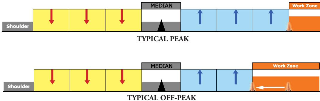
*With plastic delineation, traffic has more lanes during peak hours, and the work zone is expanded in the off-peak, but safety is compromised.*
