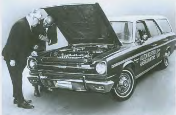
Dr. Wouk explains to New Jersey Congressman Edward Patten the function of the nickel-cadmium batteries in the power system of the Rambler.
