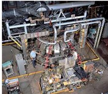
The Model C Stellarator shown in the photo on the right began operation in 1962 following a 4-½ year design and construction effort involving PPPL engineers and physicists and industrial participants. PPPL engineers converted it to a tokamak, PLT, in 1968 in a remarkably short 4 months!
