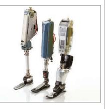
"You can say that conventional mechanical prostheses are like a bicycle and what I'm wearing is like a motorcycle-the motors actually inject mechanical energy into my walking gait, enabling me to move more efficiently," Herr said. In effect, he's tried to mimic the mechanism of a natural limb: The human spinal cord receives sensory
