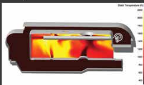
Static temperature field inside the combustion chamber of the KJ-66
