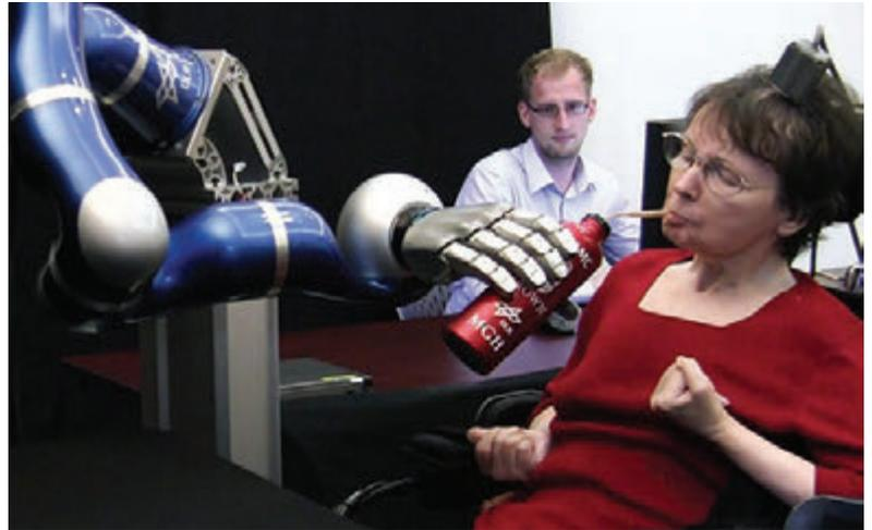
**THOUGHT INTO ACTION** A 4 millimeter square sensor (left) implanted in the brain of Cathy Hutchinson uses 96 electrodes to capture neural signals. A computer decodes the data, enabling Hutchinson, who has been paralyzed 15 years, to manipulate a robotic arm and give herself a drink of coffee.
