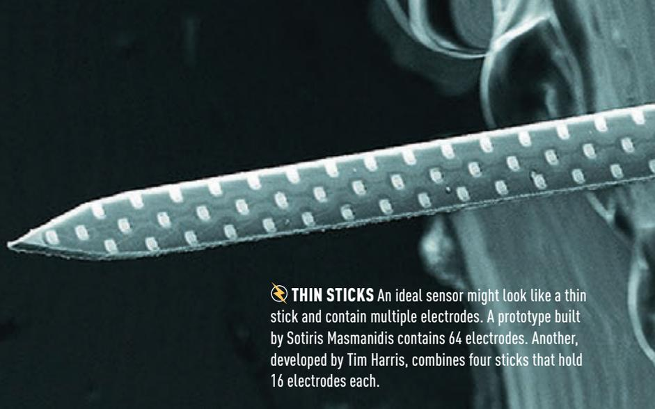
**THIN STICKS** An ideal sensor might look like a thin stick and contain multiple electrodes. A prototype built by Sotiris Masmanidis contains 64 electrodes. Another, developed by Tim Harris, combines four sticks that hold 16 electrodes each.
