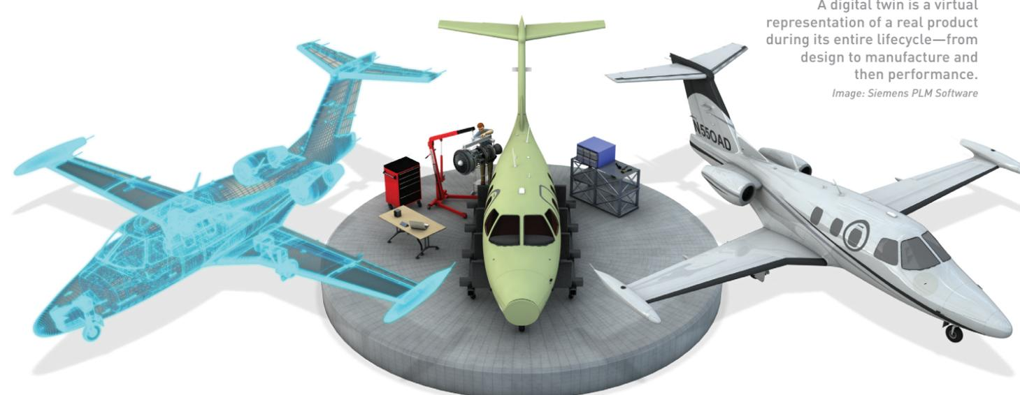
A digital twin is a virtual representation of a real product during its entire lifecycle—from design to manufacture and then performance.
