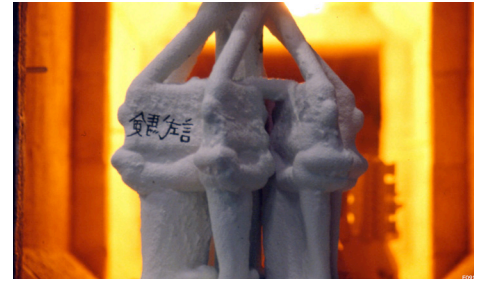
A ceramic mold for multiple directionally solidified turbine blades is placed in a vacuum furnace at Howmet's foundry in Terai, Japan.
