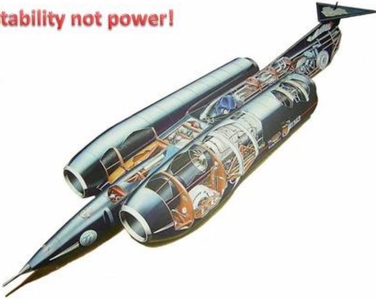
Cut-away layout drawing of ThrustSSC
