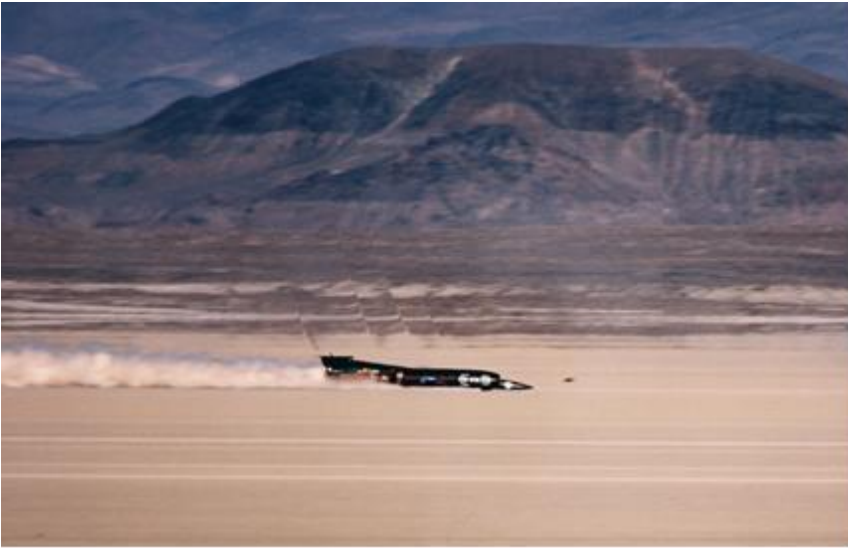
Shock waves above ThrustSSC at 763 mph
