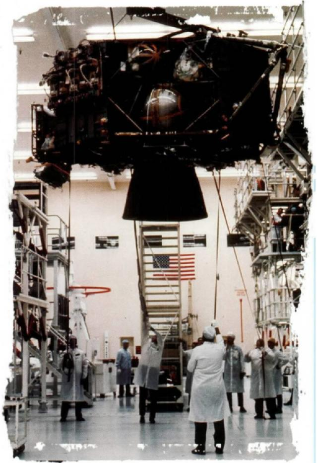
design amounted to something between the two. Because the Lunar Module would be required to perform solely in the space vacuum, engineers could ignore aerodynamic requirements associated with Earth's atmosphere. The result was an aesthetically unappealing, yet functional, spacecraft.
