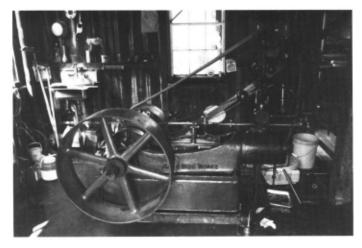
2. Cider Press - Boomer & Boschert No. 2; four 2 1/2" X 3 threads per inch power screws capable of being driven at three different speeds; 4'10" square racks with 96" square press cloths; maximum stroke of 48". Maximum capacity is approximately 10,000 pounds per day (1100 gallons). Manufactured in the mid 1890's.
