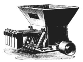
5. Cider Pump - Boomer & Boschert; bronze plunger pump, 3" cylinder with 4 1/2" stroke. Runs at not greater than 80 strokes per minute; a capacity of 10 gallons per minute. Manufactured in the mid 1890's.
