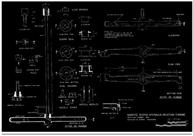
Of considerable concern was the efficiency value to be used. Since this value is a function of the nozzle and water jet velocities (and therefore the turbine angular velocity and the head of the water in the supply stand pipe) a fixed average value of 0.6 was selected for calculation purposes.
