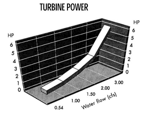
settling tank in the water channel leading to the turbine supply pipe. With the gate at the head of the water channel fully open a water flow of 0.54 cubic feet per second was measured. This was the value used for the power calculations even though there was a minor leakage through a side gate just before the turbine water supply stand pipe.
