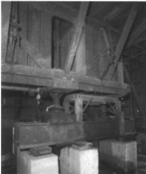
Ground floor view of the double box press which rotates on a center bearing post with hydraulic press block and cylinder under the box on the left.
