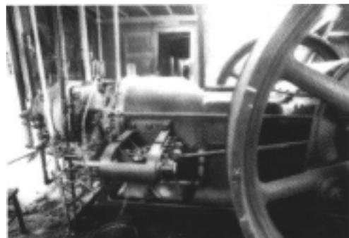
125 hp Bessemer Type IV oil engine installed in 1925.
