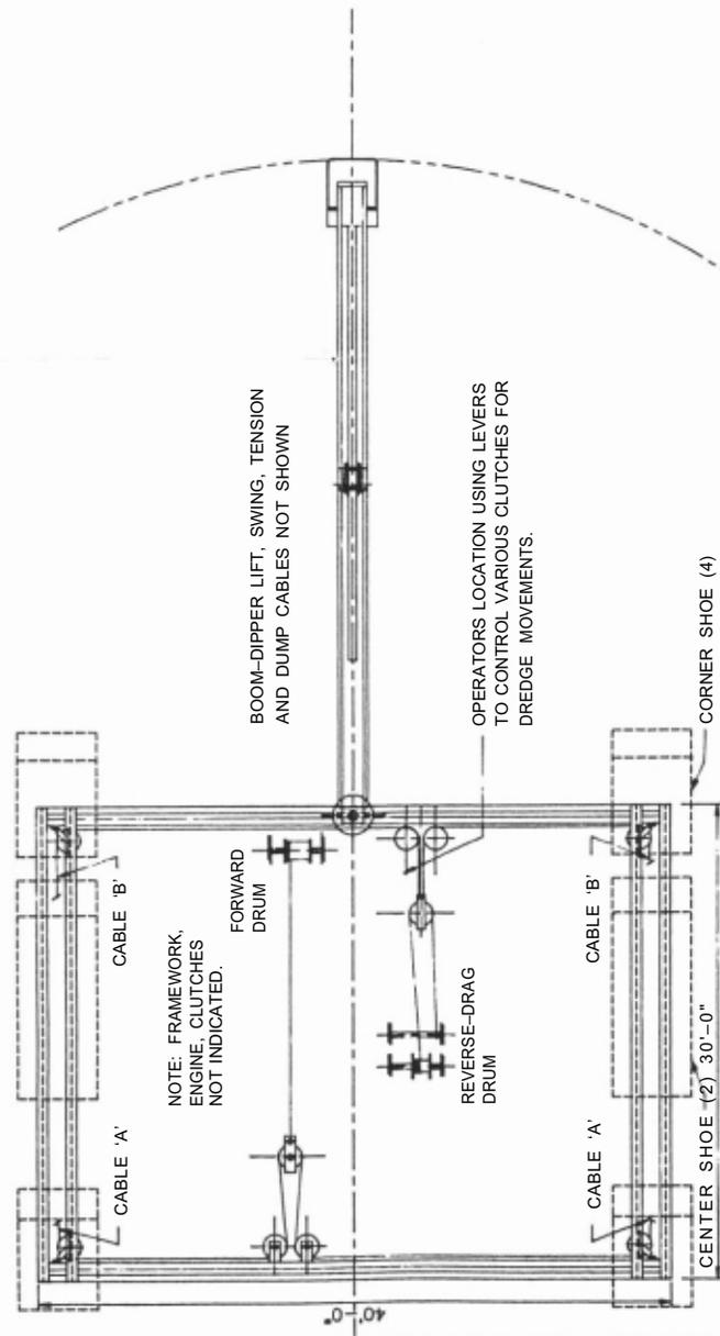
PLAN VIEW OF WALKING SHOE CABLES AND DRUMS
