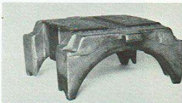
Figure 6. The AAR narrow adapter used in the modified integral box side frame and also used in the AAR narrow pedestal side frame to transfer the load from the frame to the roller bearings.
