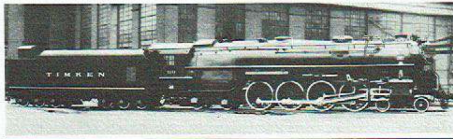
Figure 2. The Four Aces was the first steam locomotive equipped with roller bearings on all axles. It was built by American Locomotive Works in 1930 and loaned to various railroads prior to being sold to Northern Pacific in 1933.
