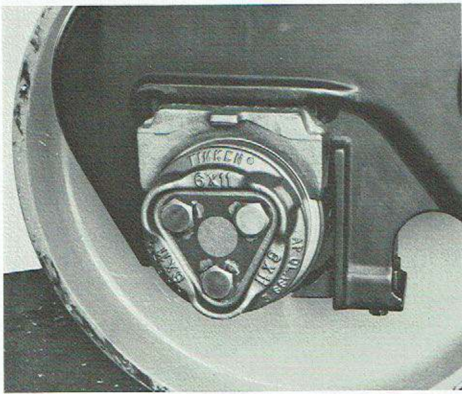
Figure 9. Front view of the AAR narrow pedestal frame with the narrow adapter and "AP" bearing.
