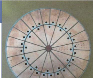
Cross section of the copper bar assembly that produces the toroidal magnetic field.
