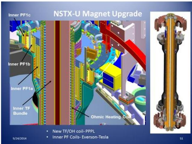
The electrical connections to the center stack are a critical area. This was an area of focus in which a number of design changes were made to accommodate the higher currents and forces of the upgrade while also improving reliability.
