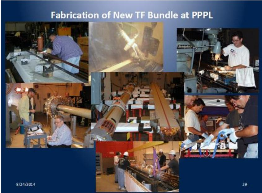
Steps to fabricate the copper bar assembly that produces the toroidal magnetic field.
