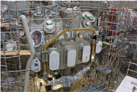
1 of 5 PPPL-supplied trim coils shown installed on W7X. [Photo courtesy of Max Planck Institute for Plasma Physics.]
