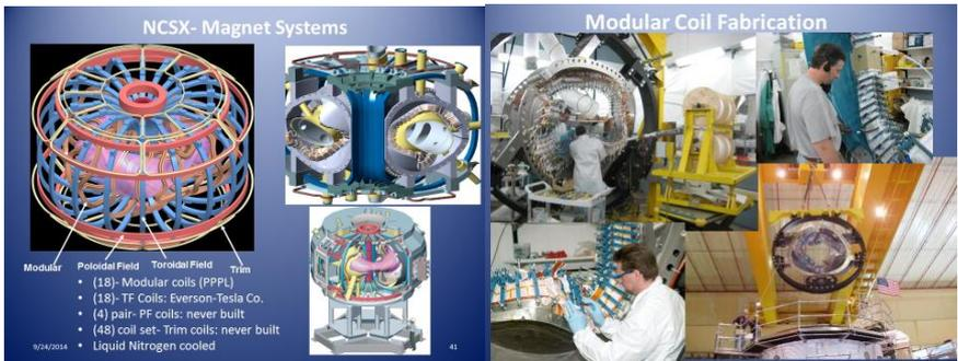
**Modular Coils Were Made to Required Accuracy**
