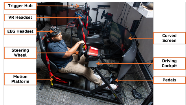
Figure 2. Key components of the driving simulator unit.
