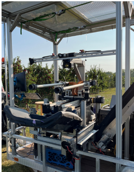
Figure 1: Prototype of the developed multi-arm apple picking robot at Li's lab.
