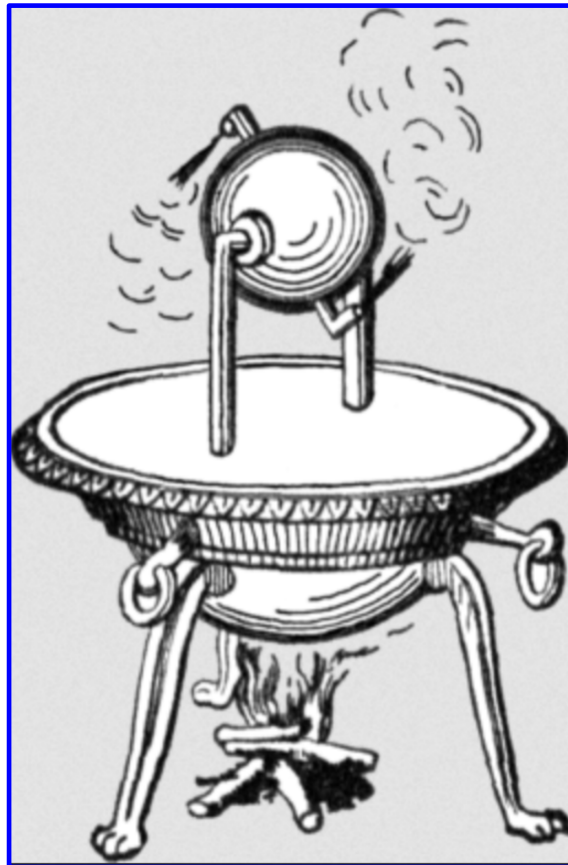
Sketch of an AEOLIPILE, invented by Hero of Alexandria (c. 10 - 70 CE)
