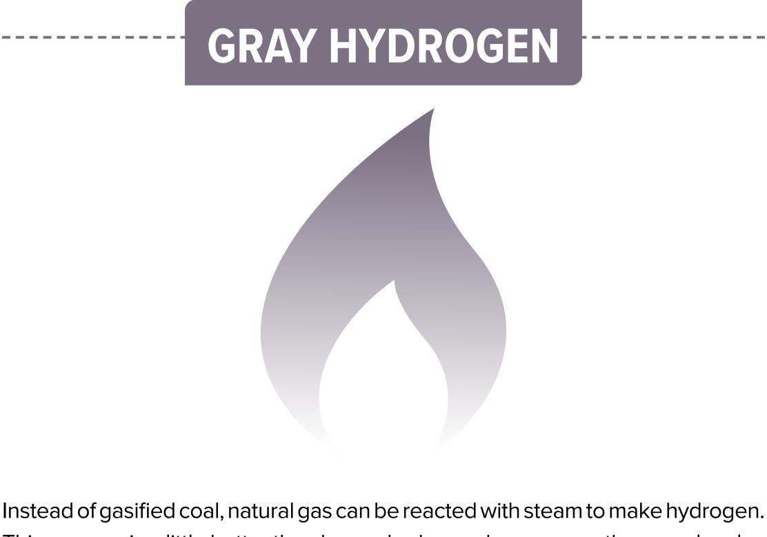
This process is a little better than brown hydrogen because methane molecules have hydrogen atoms that they can contribute, but it still results in greenhouse gases added to the atmosphere.
