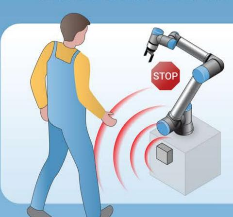
Speed and separation monitoring (SSM) provide additional precautions that can allow the cobot to exceed safety limits.
