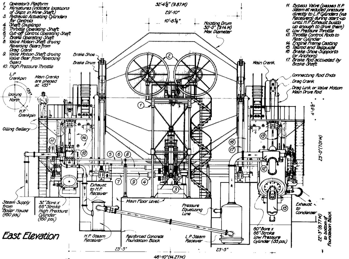
ilarly set and mounted at the opposite end of the drum shaft. The cylinder dimensions are 32" and 60" x 66".
