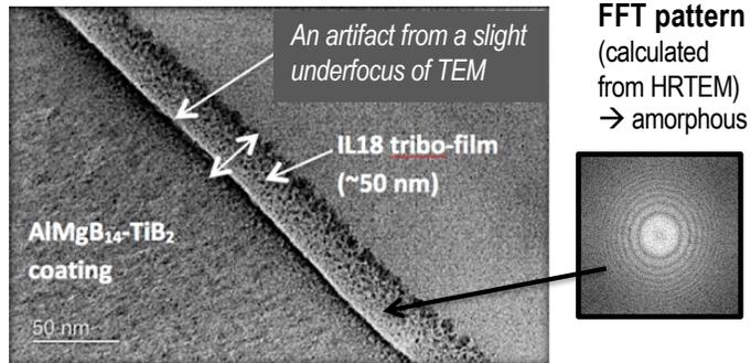
The iron-free coating surface eliminates the ambiguity of the source of Fe in the tribofilm.
