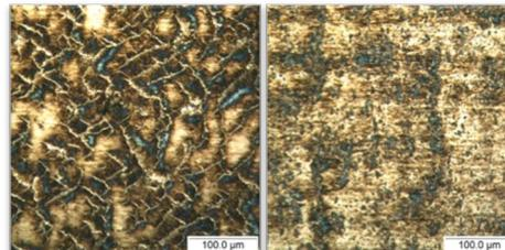
Roller surface tested in base oil
