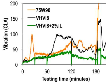
2018 Gear dynamometer tests increased 6% of the power output by using an IL-additized gear oil
