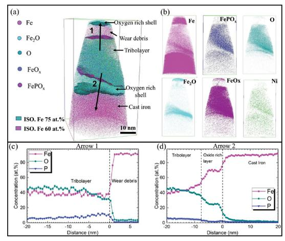
3D atom probe tomography (APT) reconstruction of the IL tribofilm showing a layered structure.
