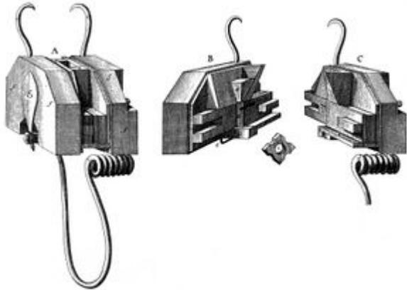
**Fig. 1.** No contemporary records exist of Gutenberg's type-making tools; he may have used molds like these 17<sup>th</sup>-century French designs.
