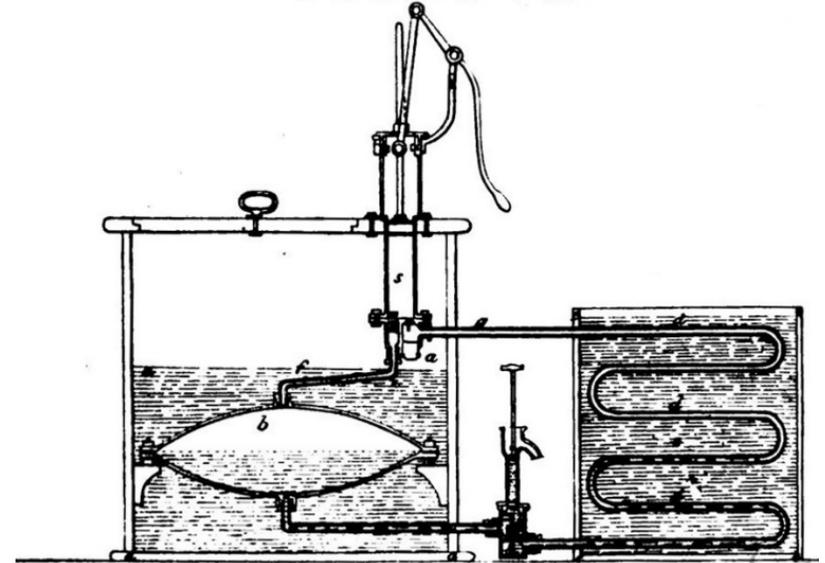
Right: Drawing from Jacob Perkin's patent entitled, “Apparatus and means for producing ice, and in cooling liquids.”
