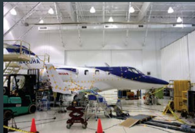
(Figure 10: Ground vibration test).
