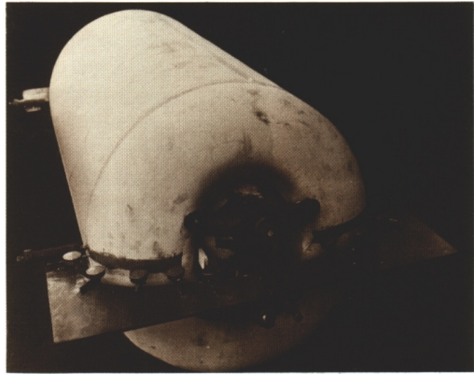
At pressures more than six times those calculated to be within safe limits, this first welded test unit was so deformed at 3250 psig that it leaked and could no longer hold more pressure.
