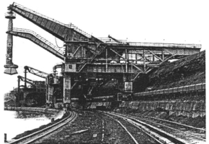
Last Hulett Built - 20 ton bucket, Lorain The Great Lakes Historical Society, Vermillion, Ohio
