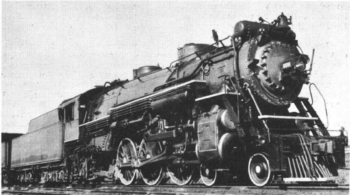
Southern Railway Ps-4 Heavy Pacific. This engine is basically a USRA heavy pacific design with a driver diameter of 72 inches instead of 80 inches for service on heavy grades.
