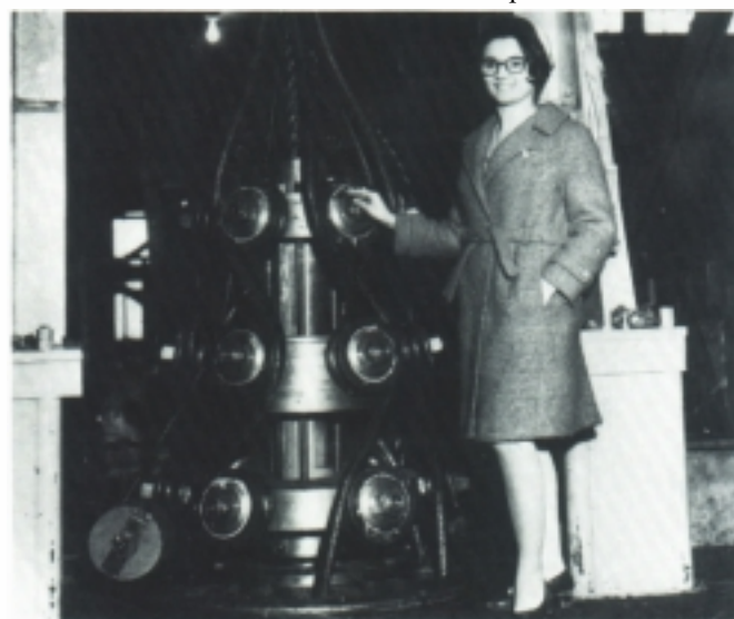
Preforming head and closing die for 5" wire rope on 80-Ton Wire Rope Machine, 1968: John A. Roebling's Sons Co. Division of Colorado Fuel & Iron Company.
