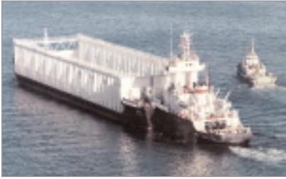
Figure 4: 6,000 HP Articouple H Tug Pushing 9,000 DWT Deck-Barge
